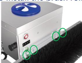
1. Hand twist combines bolt eight three fixed roller in front Kwun body with water segregator, roller without water segregator Kwun body in the rear. **(Do not tighten)**
