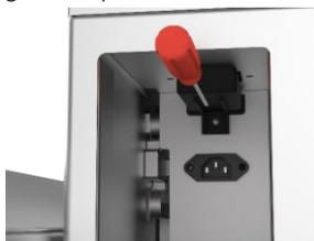
3. Take out the 4G network module, remove the cover, insert the Nano SIM card, and restore the installation.
